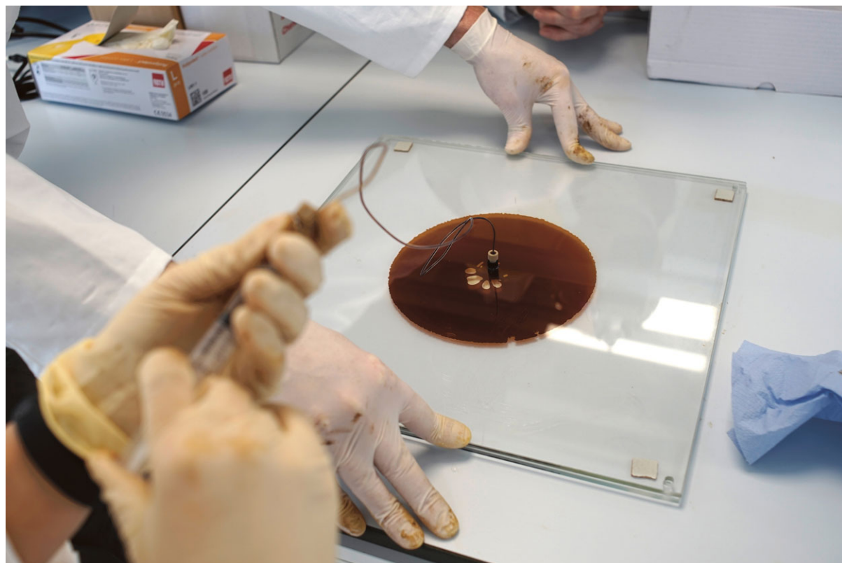
The scientific Hele-Shaw cell experiment shows how water introduced via a syringe mixes with the viscous oil. Source: Ernst Logar
